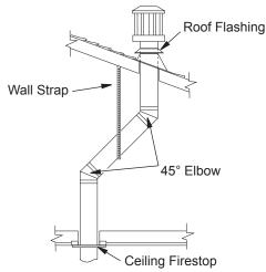
Figure 19 - Offset with Wall Strap and 45° Elbows
